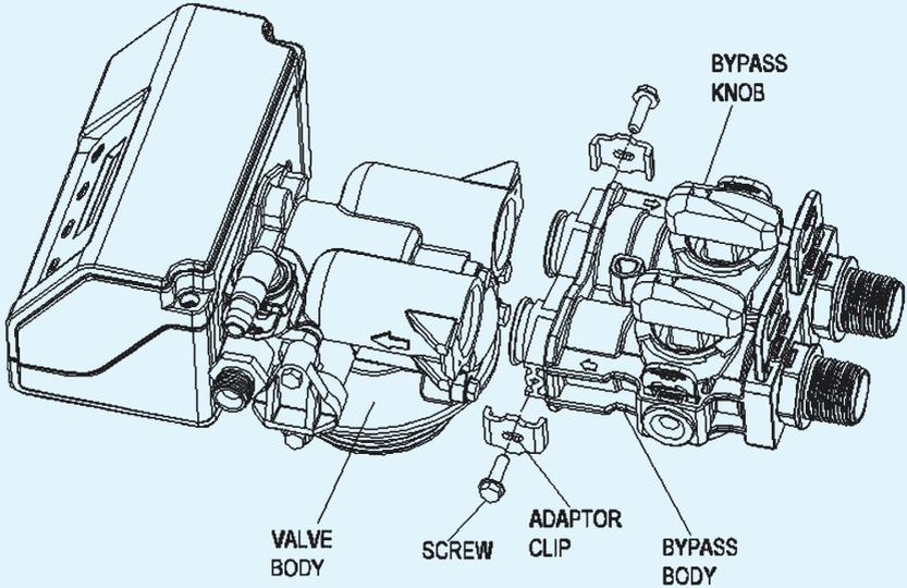
The bypass valve is provided with various functions such as bypass and water hardness adjustment. Different angles of bypass knob have different functions (see below). The larger angle (value A), the higher water hardness in hardness adjustment position.
